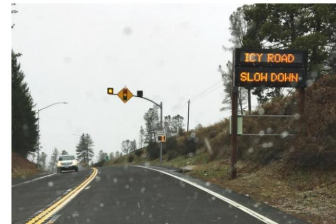
The newly improved intersection at Brunswick Road and Loma Rica Drive includes an IceSight sensor, mounted on the signal cross arm, to monitor pavement conditions. When the road surface reaches a pre-determined unsafe level, a fixed message sign warns drivers to slow down. The site's inaugural activation occurred on Sunday, 20 December 2015.
